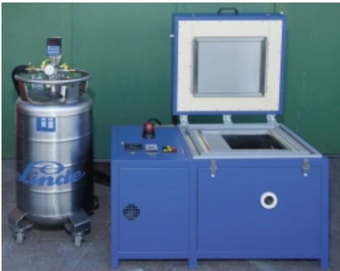
Figure 14: Liquid Nitrogen Storage in Nitrogen Dewars Holds Typically 50 Liters (100 Gallons) of LIN
